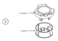
Separate the holder and the mesh by pinching one side of the mesh and pulling.
