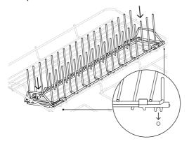
Align front and rear clips with the base rack and clip into place.
