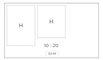
If there is a power interruption while the residual heat indicator is active, the cooktop will restart at residual heat temperature with 'H' displayed on the touchscreen.
