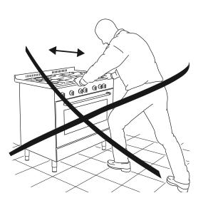
To restrain the range and prevent it tipping accidentally secure the range to the wall using the supplied anti-tip bracket. Ensure you also fit the supplied lock pin to the anti-tip bracket.
