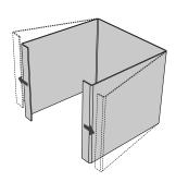
③ Gently bend the edges of the inner cover to adjust the tension between the two parts if needed.
