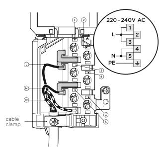
② Unscrew the screw to open the cable clamp. For OR90SCG6 and OR90SDG6 models, connect the U bolts onto the terminal.
