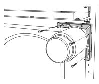
① Tip range onto its back and fix brackets to mounting holes.
