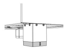
6 Adjust the inner panels of the foot covers to suit height of range feet.
