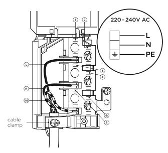
3 Connect the phase, neutral and earth wires to the terminal board as shown. Strain the feeder cable and block it with cable clamp. Screw clamp shut before closing the main cover.
