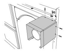
4 Secure covers to brackets using the provided screws
