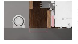
Push the toe kick back to the desired depth before removing. If toe kick depth is less than 90mm, attach the additional foam block.
