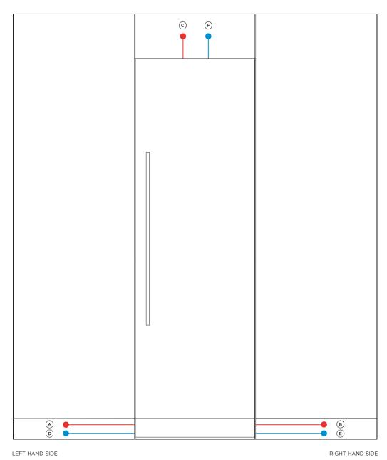
Specifications Electrical Supply 230 VAC, 50 Hz Service 10 amp circuit Plumbing Supply Water Filter UK IE SG HK Braided hose, 7/16" x 24 UNS to 3/4" BSP NZ AU Braided hose, 7/16" x 24 UNS TO 1/2" BSP Pressure min 275 kPa (40 psi) max 827 kPa (120 psi)
