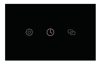
4. Press ① to start or stop DELAYED OFF timer. Press and hold to adjust delay duration. If LINK MODE is on, timer will start when linked zones are turned off.
