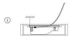
Connect one end of the suction tube to the large adapter attached to the suction inlet in the vacuum tank.
