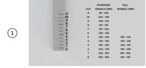
Measure the distance between the floor and the base of the door. Refer to the table and mark out the cut location. Score at the marked height, snap off excess material and smooth edges.
