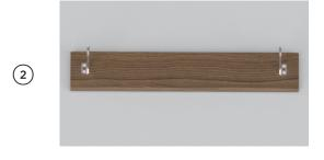
Ensure brackets are oriented correctly before fitting to the panel using 2 x screws per bracket.
