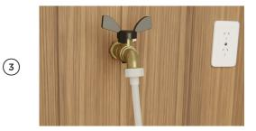
Ensure the rubber washer is fitted when connecting the inlet hose to the tap. Hand-tighten into place.
