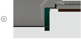
Align both sound seal sheets to the base of the dishwasher. If required, trim excess felt.
