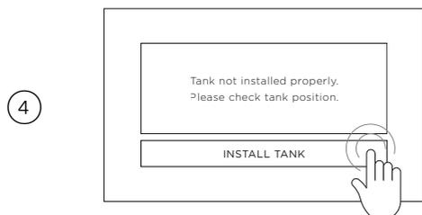
If the tank is incorrectly re-installed or the water level is too low, follow the onscreen guidance before continuing.
