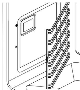
Slide the side rack forward until the rear tabs are clear of the mounting studs.
