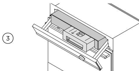
When prompted, press the touch screen to open the control panel. Pull water tank out and fill to the **MAX** fill line.
