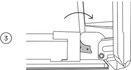
Ensure the levers are both fully locked before trying to shut the door.
