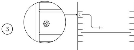
Place food in the oven and plug the probe into the socket inside the oven, on the left hand side.
