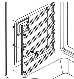
Unscrew and remove the fixing nut at the front of the side rack. Use a coin to loosen the nut if necessary.
