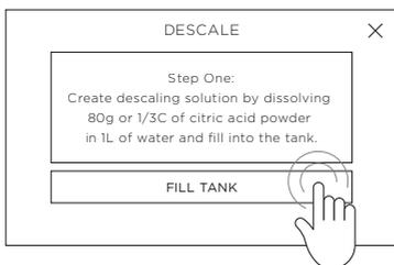
Fill tank with 1L of descaling solution\* and select **FILL TANK** to begin process.
