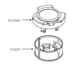
Separate the holder and the mesh by pinching one side of the mesh and pulling.
