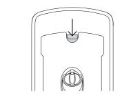
Press the latch down to open the dispenser. Check that the dispenser is empty and dry.
