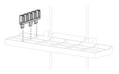
This clips onto the adjustable racks and supports knives and other utensils during the wash.
