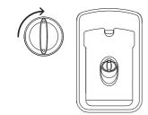
Refit the cap, turning clockwise until secure.
