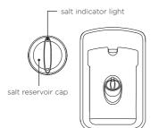
The salt reservoir is located on the inside of each drawer next to the detergent dispenser. It holds up to approximately 350g of salt (actual capacity will vary depending on brand and grain size of salt used).
