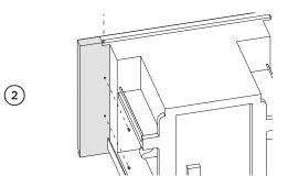
Attach the side trims using the hex key and 6 of the screws provided. Do not over-tighten.
