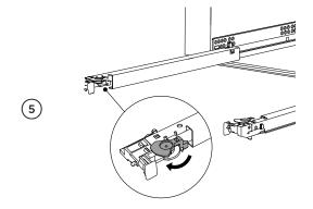
Use the levers at the front of the rails to adjust the height of the appliance.
