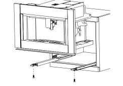
Position the appliance on the rails, making sure the pins are correctly inserted in the housings, then fix it with the screws supplied.
