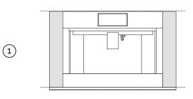
Align the side trims on either side of the coffee maker, using the locating tabs and corresponding slots.
