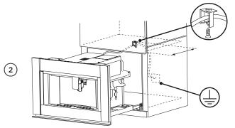
Fix the power cable with the clip. The power cable must be long enough to allow the appliance to be extracted from the cabinet to fill the coffee bean container.
