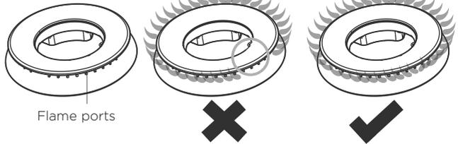
Burner parts may not have been replaced correctly. Check the assembly and make sure the burner cap and/or ring is sitting flat on the flame spreader. See 'Care and cleaning' for illustrations.
