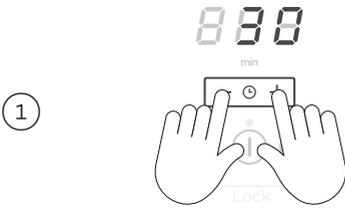
With the cooktop turned on, tap the - and + controls together until the indicator light in the desired cooking zone illuminates.
