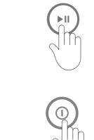
To stop the dryer at any point during the WRINKLE FREE stage of the cycle, press ▶II. You can then open the dryer door and remove your items.
