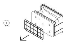
Remove the bracket securing the foam to condenser filter.
