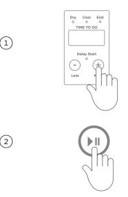
Press MORE + to increase the delay time, and LESS - to decrease the time, or turn DELAY START off.
