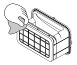
Use your hand, a cloth or a vacuum with a crevice nozzle to remove any lint build-up from the mesh surface of the filter.
