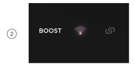
Press and hold Wi-Fi button for 5 seconds until it flashes, or open the app and remove rangehood.
