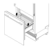
Lower the front end of the steel bin ensuring the sides are sitting on the sliders.
