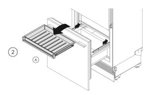
Remove the mid tray (A) and retract the sliders.
