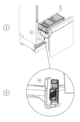
To remove a bin, extend the bin on its runners ((), and empty the bin.
