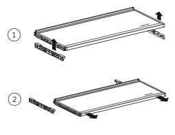
To remove, hold the front and back edge of the shelf firmly.
