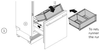
To return the bin, extend the runners and place the bin on top of the runners (()).
