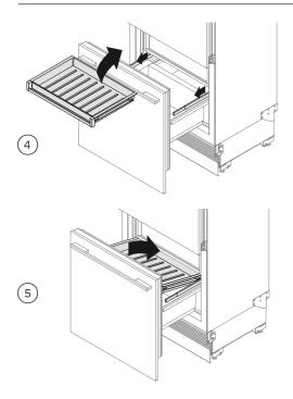
Pull out the sliders and insert the rear end of the mid tray into the appliance
