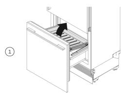
Open the bottom drawer fully. Unclip the mid tray from the sliders and lift the front of the tray.
