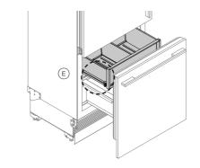
Push the bin slowly onto the securing tabs until you feel it clip onto the runners (E).
