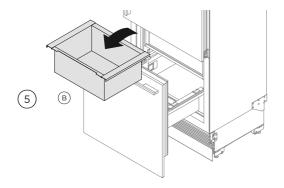
Lift the steel bin (<sup>®</sup>) upward to remove.
