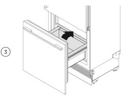
Lift the steel bin slightly and slide back inside the appliance to unseat the steel bin from seating pockets.
