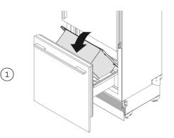
Open the bottom drawer fully. Insert the rear end of the steel bin at an angle into the bottom drawer.
