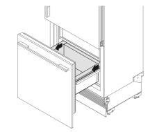
Slide the steel bin slightly forward to locate into the seating pockets.
