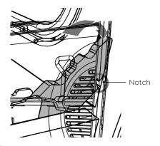
② Insert the hinge tongues into the slots, making sure that the notches on both sides drop into place as shown.
