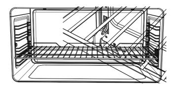
4 Lower the shelf back onto the side rack wires and slide all the way into the oven.
