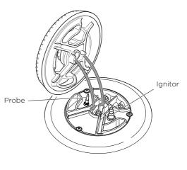
Correct positioning of cap and ring - triple-ring wok and dual burner
