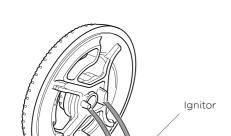
Correct positioning of flame spreader -dual burner
