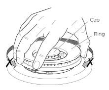
Incorrect and correct positioning of cap and ring - triple-ring wok and dual burner
