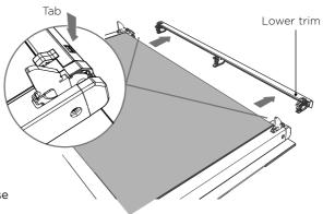
③ Press down on the tabs to release the lower trim and remove it.
