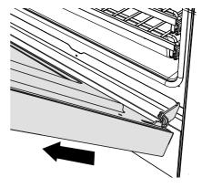
4 Disengage the hinges and remove the door. Place on a protected surface.
