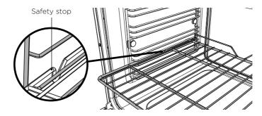
3 Tilt the front up slightly to help the safety stops clear the side rack wires.
