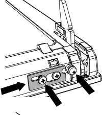
® Re-tighten the screws so that the latches and the lower trim are firmly secured.
