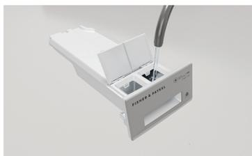
To clean the dispenser drawer, fill the compartments with warm water and shake lightly to clear residue. Drain all water from the compartments before refitting the dispenser drawer to the washer.
