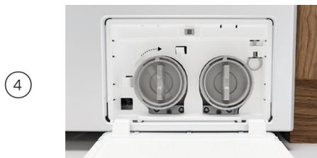
4 Refit the filters and turn clockwise to secure. The handles should be in the vertical position. Do not use excessive force to tighten.
