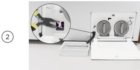
2 Unhook the outlet hose and pull it out (approximately 150mm). Remove the plug and allow any water to drain into a shallow dish (approximately 250ml).
