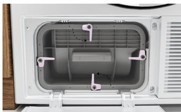
Turn the four condenser lock levers 90° then pull out the condenser filter.
