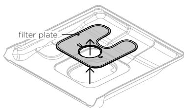
With the filter removed, carefully lift the filter plate up and out.
