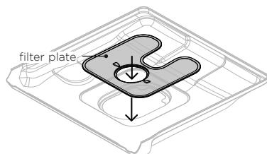
Slot the filter plate under the locating clips at the rear of the drain and push firmly back into place. Ensure the filter plate is flush with the dishwasher base.
