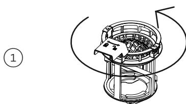
Twist the filter anti-clockwise to release.
