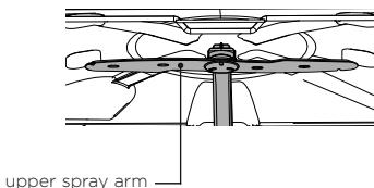
Do not remove the upper spray arm for cleaning. Clean with a small, plastic-bristled brush. If heavily soiled or blocked use a dishwasher cleaner/descaler. Follow the manufacturer's instructions.
