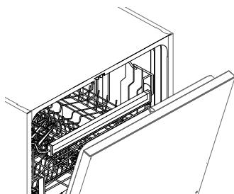
After the wash the door will automatically open slightly to assist with drying.\*
