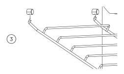
Swing the bottom of the side rack up towards the center of the oven until it is almost horizontal. Slide the prongs at the top out of the mounting slots.
