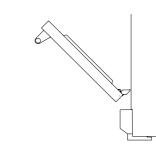
Holding the door at 45°, carefully align the hinge tongues with the hinge slots. Push the door in until you feel the latches locate into position on each side
