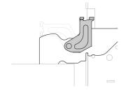
Rotate the locks up into the closed position ensuring they rest inside the slots completely. Note: Incorrect installation will prevent door from correctly sealing.
