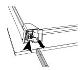
4 Holding the door on both sides, line up the holes in the base of the door with the hinges and slide the door on.
