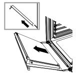
③ Holding the door on both sides, lift door back up to 45° and carefully pull the door out and away from the hinges.
