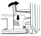
(6) IMPORTANT! Ensure the levers are both fully locked before trying to shut the door.
