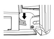
(5) Ensure the door is firmly in place on the hinges. Open the door fully again and push each locking lever down to lock the door onto the hinge.
