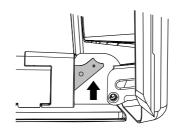
② Push each locking lever up fully to release the door from the hinge.
