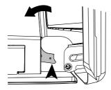
Open the door fully. Locate the two small metal locking levers on both door hinges either side.
