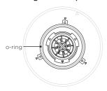
Before refitting the filter plate, ensure the O-ring is correctly positioned in the tub as shown.
