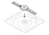
Place the spray arm onto the impeller. Ensure that the arm rotates freely when refitted.
