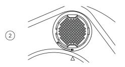
Place the filter back into the tub by aligning the arrow to the  $\widehat{\Box}$  on the filter. Rotate clockwise until the arrow aligns with  $\widehat{\Box}$  and clicks into position.
