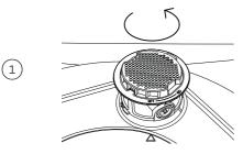
Twist the filter counter-clockwise until the arrow in the tub points to  $\widehat{\ }$  on the filter. Lift to remove.
