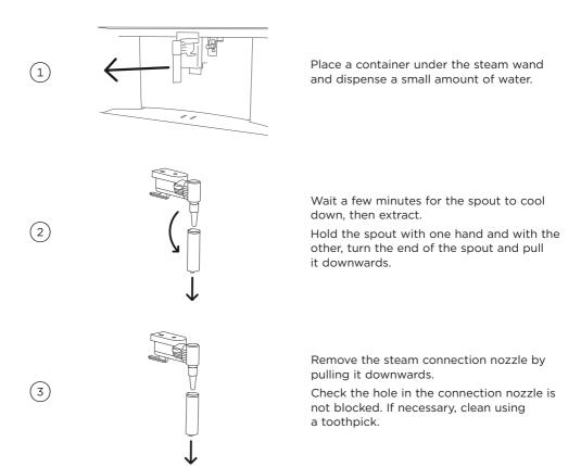
Replace all components. Insert the steam connection nozzle, then the steam wand spout by pushing it upwards and turning it clockwise until firmly in place.
