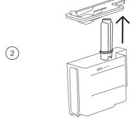
Follow the instructions on the screen. Remove the water tank and water filter (if fitted) and empty.
