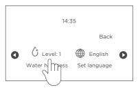
To change the level selected, touch **WATER HARDNESS** until the required level is displayed.
