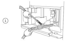
If necessary, remove coffee deposits with the brush supplied and a sponge. Remove remaining residue with a vacuum cleaner.
