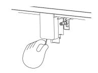
Check that the holes in the coffee spouts are not blocked. If necessary, remove coffee deposits with a toothpick.
