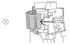
After cleaning, replace the infuser by sliding it onto the internal support and pin at the bottom, then push the PUSH symbol fully in until it clicks into place.
