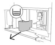
Remove the grounds container, empty and clean. Ensure all coffee residue is removed, using the spatula or the brush provided.
