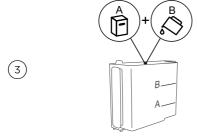
Add descaling solution to the water tank, following the instructions on the screen. Place water tank back in the appliance.
