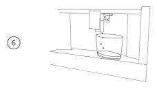
Place a container underneath the steam wand to catch any water.
