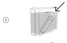
Remove the water tank and fill with fresh water. Place the filter in the tank, immersing completely for about ten seconds.
