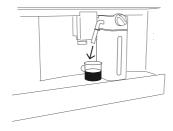
Fill the milk container and attach it. Position the cup under both the coffee dispenser and the milk spout.
