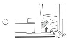
Push each locking lever up fully to release the door from the hinge.
