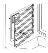
Fit the side rack front tab over the fixing screw.
