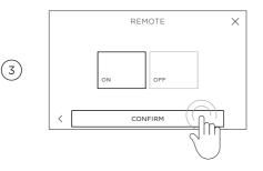
Select ON then press CONFIRM. REMOTE MODE is now enabled. This setting is designed for religious faiths that observe a 'no work' requirement on the Sabbath.
