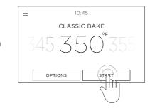
To adjust the preset temperature, swipe left or right or use the dial. Touch **START** to heat the oven and begin cooking.
