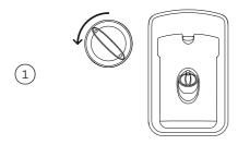
Turn the cap anticlockwise and remove.
