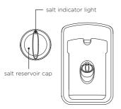
The salt reservoir is located on the inside of the drawer next to the detergent dispenser. It holds up to approximately 0.8lb (350g) of salt (actual capacity will vary depending on brand and grain size of salt used).
