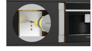
Fit the bracket into place using the supplied screws. Repeat on opposite side.
