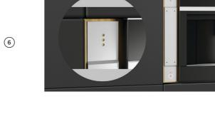
Ensure the top and bottom of the bracket sit flat against the cabinet. Align with the pilot holes.
