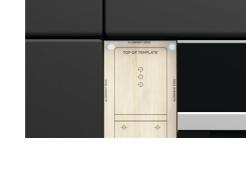
Ensure the template is completely flush against the cabinet and all four coners are secure.
