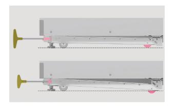
1. Open the cabinet door and lower the rear wheel using the supplied Allen key.
