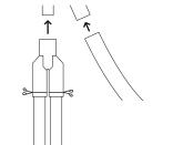
Install your Air Gap Kit to the benchtop. We recommend using a Dual Air Gap Kit. Refer to 'Plumbing & electrical connection' for minimum install heights.
