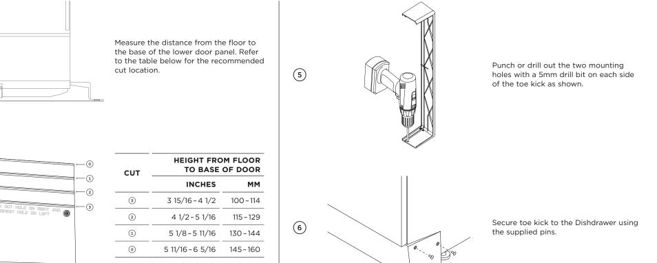
\*recommendations are based on the required min. clearance of 12mm between the floor and toe kick
