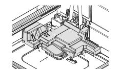
Refit module cover before sliding the access cover back into place, ensuring the 2 clips shown are fully locked.
