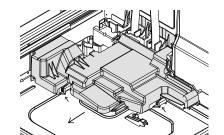
With a flat-bladed screwdriver, push in the clips and slide out the access cover.
