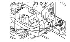
Screw down the Live, Neutral and Earth wires correctly.
