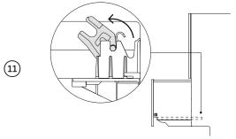
Before refitting the drawers, ensure the hoses are not twisted and all latches are facing forward.
