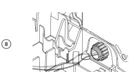
Safely cut the cord from the inside **and outside** of the product to remove the cord.
