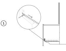
Open the lower drawer and press both locking tabs back to release.
