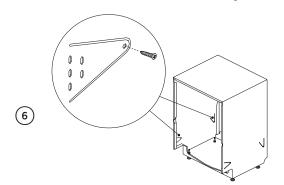
Using your hand or the supplied hex socket and a screwdriver, level the DishDrawer™ Dishwasher as required. Rotate clockwise to increase the height of each leg and anticlockwise to lower.
