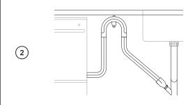
clips on to the hoses and fitting to the supplied hose joiner. Secure using the wire clips. Ensure hose is routed straight to the joiner, removing excess drain hose if
