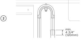
Pull both hoses through the support guide and rest in standpipe.
