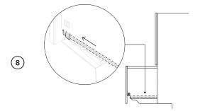
Before refitting the drawers, ensure the hoses are not twisted and all latches are facing forward.
