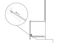
Refit the drawer back onto the runners, ensure both runners are entended halfway before lowering the tub. Slide the runners forward to engage.
