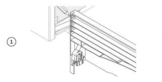
Measure toe kick height. Where the toe kick meets the bottom of the tub is the recommended cut-off point.
