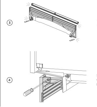
Snap excess + smooth edges. Snap both end tabs.
