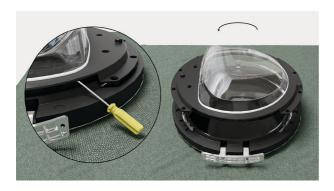
2. Insert flathead screwdriver in access slot to pry off inner door. Rotate door 180 degrees and fit back in place.
