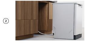
Push the product into the position, pulling the hoses through as you push to avoid crushing or twisting them. Take care not to bend the legs.
