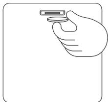
Turn the power off and unplug the washer. Use a coin to open the filter cover. Place the edge of the coin into the slot and tilt upwards whilst levering the cover open.
