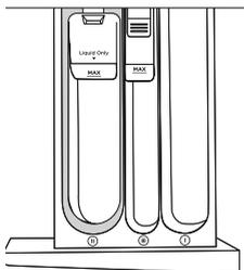
Detergent is added to the main wash compartment on the left side of the dispenser drawer marked with a **II**.
