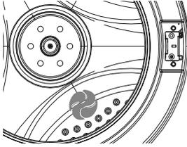
Detergent pods are a no mess alternative to powdered or liquid detergent. They must be placed at the back of the drum prior to loading your clothes. This will ensure they are activated quickly in the wash. Do not place pods in the detergent dispenser drawer or on top of your clothes.
