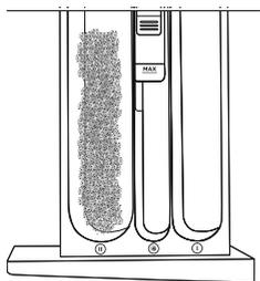
Detergent is added to the main wash detergent compartment on the left side of the dispensing drawer marked with a (II).
