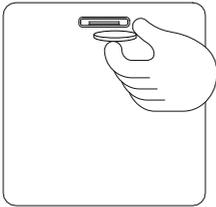
Place a coin or key in the slot and tilt it upwards to lever the cover open.
