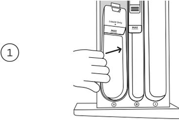
To remove the liquid detergent compartment, firmly grasp and twist the left hand side of the internal compartment and pull upwards.
