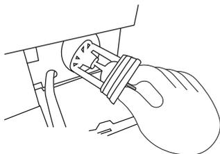
Remove the filter by turning anti-clockwise. Clean and rinse under a tap. Check the pump filter cavity for any further obstruction.
