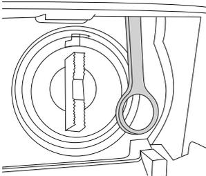
Pull the door release tab down from the ring. Use a screwdriver tip, pen or key to get a good grip.
