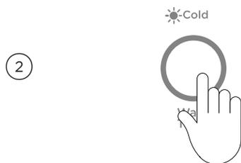
The cold **WASH TEMP** icon will flash on and off. This is the default setting, where the machine uses the internal heater to heat the water to 20°C.
