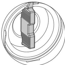
Replace the filter by turning clockwise until the turning handle stops in the vertical position, and cannot be turned further.
