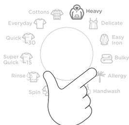
Select your desired wash cycle by turning the Control Dial. The wash cycle icons will illuminate as you turn the dial showing which cycle is selected, along with the default wash cycle settings.
