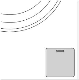
Locate the pump filter cover at the bottom right of your washer.
