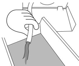
Unhook the pump outlet hose and pull it out (about 150mm). Remove the plug and allow any water (approximately 250ml) to drain into a shallow dish.
