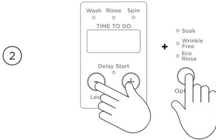
Press **MORE +**, **LESS -** and **OPTIONS** buttons together for three seconds, *dEF* will appear on the screen and the washer will beep.
