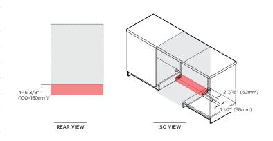
Service outlet at rear extends both sides, hoses and cords can be routed to either or both sides. \*Depending on adjustment of leveling feet.
