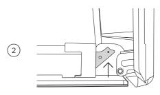
Push each locking lever up fully to release the door from the hinge.
