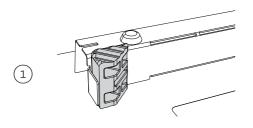
Ensure the rubber stoppers are still attached at the top of the pane. Ensure they are positioned correctly on the glass with the longer side running down the side of the glass pane.
