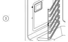
Slide the side rack forward until the rear prongs are clear of the holes.
