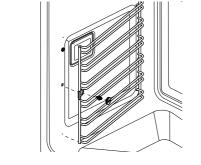
Fit the side rack front tab over the fixing screw.
