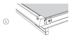
Push the glass retainer tabs in on both sides of the door again. The glass retainer can then be pulled off completely. Gently pull the middle pane toward the top of the door until the pane is clear of the notch at the bottom of the door.
