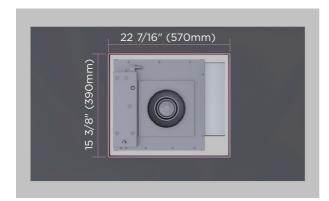
2. Create a 22 7/16" x 15 3/8" (570 x 390mm) cutout in the base of the cavity for the external blower.
