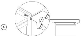
Secure to cabinetry via the brackets. Pre-drilling a pilot hole may be required depending on the cabinetry material.
