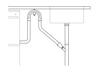
Pull the hose through the drain hose support before threading the wire clip on to the hose and fitting to the supplied hose joiner. Secure using the wire clips.
