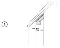
Align the supplied moisture protection tape to the cabinetry as illustrated
