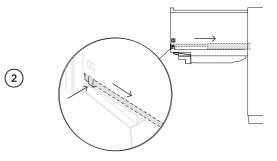
Open the drawer and press both locking tabs back to release.
