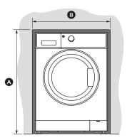
Cut out dimensions above are to be used as **minimum** dimensions.
