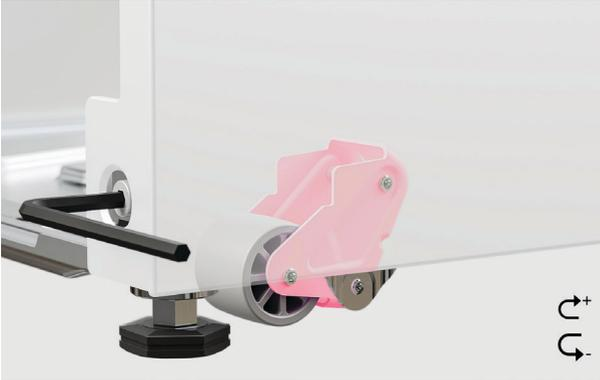
1. Partially roll stacked products into alcove and check alignment. To do this, use the supplied 6mm hex key, rotate clockwise to lower both sets of wheels via the adjustment screws.
