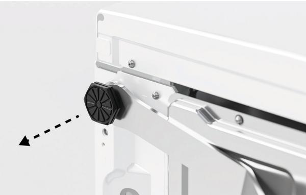
2. Unwind feet using the supplied spanner to remove.
