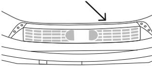
Locate the metal sensors just behind the lint filter.
