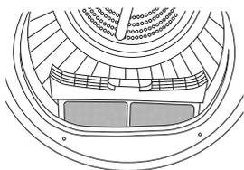
The door lint filter is located in the door opening (at the bottom).
