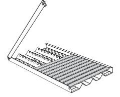
④ Place the 18 ceramic rods onto the radiant.
