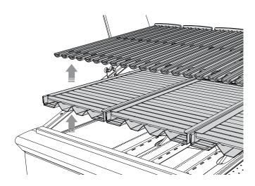
① Remove grates and radiant trays from inside the burner box.
