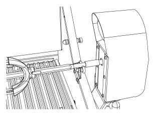
Place prepared rod into motor, lay across and into the rollers on other side.
