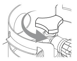
③ Open the LP tank valve. (Two full turns min).
