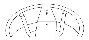
② Once located, secure to the bottom of the island using all eight hole locations provided on the restraint. Wood screws can be used for wooden floors or 1/4 inch diameter anchor screws or bolts may be used if the floor is concrete or masonry.
