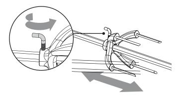
Determine the center placement for the food, put first prong on the rod, turn "L"-shaped screw to tighten.
