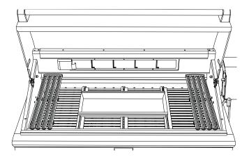
④ Remove grates and top rack on the grill. Place bottom portion of broiler pan on ceramic rods so meat drippings can be caught in pan.
