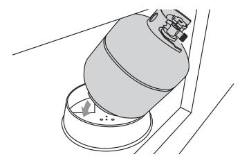
③ When secure, place the LP cylinder into the tank restraint making sure to seat the tank all the way down, securely affixing the tank in the restraint.
