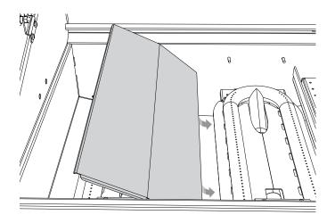
3 Lower the heat shield down between the two burners and tilt up to lay flat at the base of the burner box.
