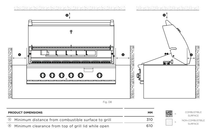
\*\***DEFINITION OF COMBUSTIBLE MATERIAL** - Any materials of a building structure or decorative structure made of wood, compressed paper, plant fibers, vinyl/plastic or other materials that are capable of transferring heat or being ignited and burned. Such material shall be considered combustible even though flame-proofed, fire-retardant treated or surface-painted, or plastered.
