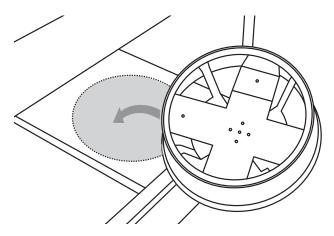
Place the tank restraint in the island and locate within the recommended area.
