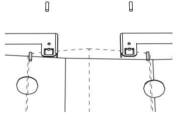
② Locate the four resting pins (two on the back wall underneath the burner hangers and two opposite at the front of the burner box).
