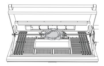
Once placement has been verified, ignite burner and start rotisserie motor. Keep on "HI" for cooking all meats on the rotisserie.
