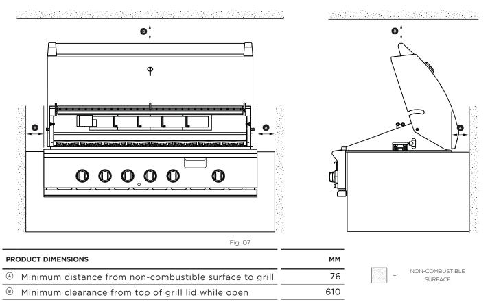
\*DEFINITION OF NON-COMBUSTIBLE MATERIAL - Material which is not capable of being ignited and burned, such as materials consisting entirely of, or a combination of, steel, iron, brick tile, concrete, slate, and plaster.
