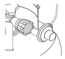
Attach regulator hose assembly to the tank.
