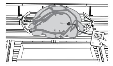
③ To check temperature of the meat, turn off motor and turn temperature to low while using a meat probe. Poultry should read 75°C in the breast. Thermometer should touch the breastbone, then lift up 2 cm from the bone to get a more accurate temperature reading.
