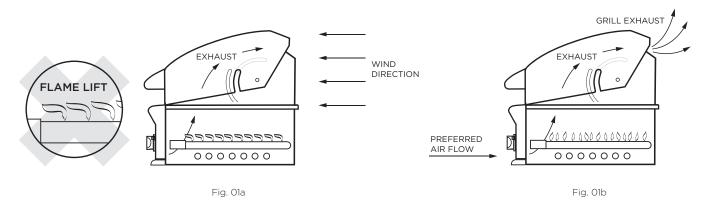
Wind hitting the grill while in use (especially wind blowing into or across the hood gap) can cause poor performance and in some cases can cause the control panel to get dangerously hot.
