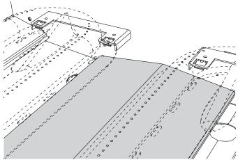
Lift and guide the shields corners to rest on the four pins located in step 2.
