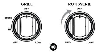
④ Once finished, turn the motor and rotisserie knob to "OFF". If you have finished using the appliance altogether, turn the main gas supply off too.
