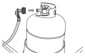
Attach the regulator hose assembly and operate the grill normally as described in the manual.
