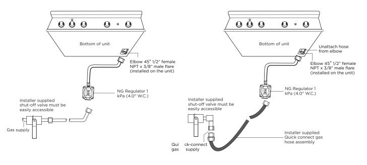
Fig. 11a - Connection with rigid piping
