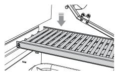
Place the assembled radiant into the unit.
