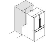
Roll the refrigerator into its final position ensuring there is the correct air gap between the product and surrounding cabinetry. See minimum clearance in cabinetry dimensions table.
