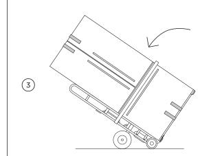
Tilt backward to load appliance onto hand truck and push to install location.
