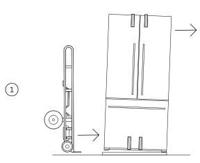
Tilt the appliance slightly forward and Insert the hand truck between pallet and appliance.
