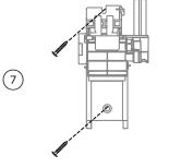
Attach the wall mounting bracket with the two screws provided, attach the bottom screw first then the top screw.
