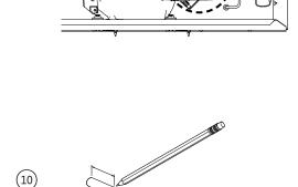
Measure 5/8" (16mm) from one end of outlet tubing and mark a line.
