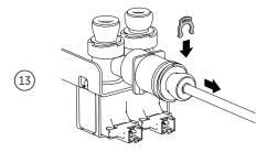
Insert a locking ring and then pull the outlet tubing gently to ensure it is locked.
