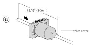
Insert one end of the outlet tubing into the tube bore of the water valve cover and slide back about 1 3/16" (30mm).
