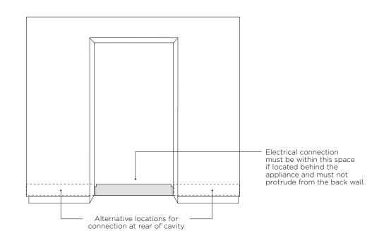
We recommend the use of an isolating switch that is easily accessible to the user after the refrigerator is installed.
