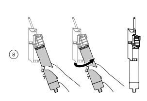
Insert the filter water into the filter head. Push the filter firmly into the filter head and turn in a clockwise direction until it locks into place.
