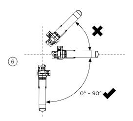
Determine the mounting position for the water filter noting the following:
