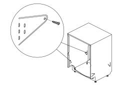
Secure to cabinetry via all four fixing locations in the chassis.
