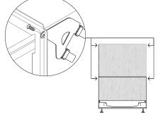
Secure to cabinetry via the brackets. Pre-drilling a pilot hole may be required depending on the cabinetry material.
