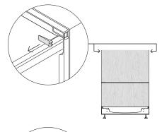
Partially open one of the drawers and remove the first screw cover from the trim moulding.
