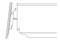
Carefully fit the panels onto the product. When refitting the lower panel, we recommend pushing back the drawer slides as shown on page 13 for access.
