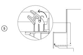
Before refitting the drawers, ensure the hoses are not twisted and all latches are facing forward.
