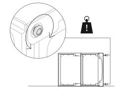
Level the DishDrawer™ Dishwasher by carefully tipping it onto protected surface.
