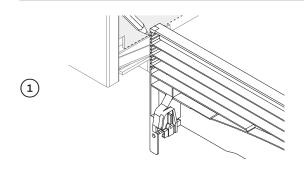
Measure toe kick height. Where the toe kick meets the bottom of the tub is the recommended cut-off point.
