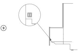
Re-insert the side pins on both drawers and push firmly to secure panels in place.
