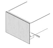
Insert a Phillips screwdriver into the hole above each side pin and rotate to adjust the panel alignment. There is a maximum travel distance of ± 2mm.
