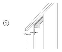
Align the supplied moisture protection tape to the cabinetry as illustrated
