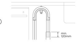
Pull both hoses through the support guide and rest in standpipe.
