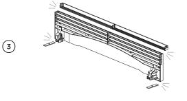
Snap excess + smooth edges. Snap both end tabs.
