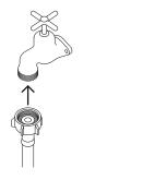
Ensure the supplied rubber washer is fitted to the coupling before connecting the inlet hose to tap. Hand-tighten into place.
