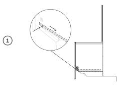
Open the lower drawer and press both locking tabs back to release.
