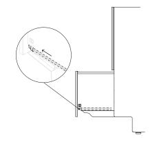
Refit the drawer to the runners and clip into place via both locking tabs.
