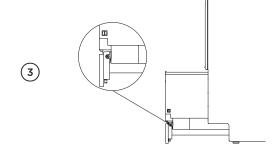
Slide toe kick onto the mounting rails and secure
