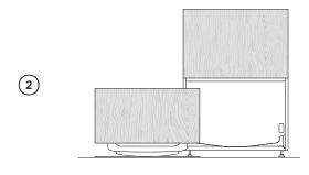
Lift the drawer off the runners and carefully set aside on a protected surface. Push runners back in.
