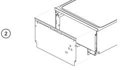
Carefully pull both brackets from DishDrawer™ Dishwasher down and out before unplugging the Knock-to-Pause modules and earth wires.
