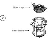
Separate the filter cap from the base by pressing the release buttons and lifting.
