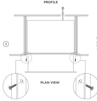
Open the drawer and secure the attachment flanges of the drawer to the side edges of cabinetry with T20 star head machine screws.
