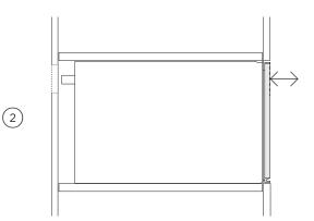
The front panel depth is adjustable within 4mm.
