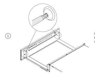
Open the drawer fully, and slightly loosen the T20 star head machine screws.
