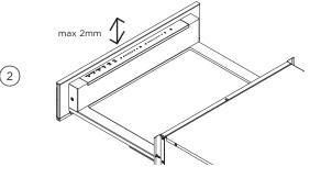
Adjust to the required height and then re-tighten the screws. The height is adjustable within 2mm.
