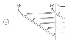
Supporting the side rack from underneath, hold it almost horizontally and locate the prongs into the mounting slots.
