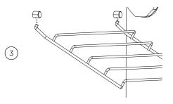
Swing the bottom of the side rack up towards the center of the oven until it is almost horizontal. Slide the prongs at the top out of the mounting slots. Refitting the side racks - secondary cavity
