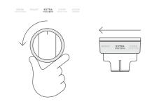
Set the oven to **EXTRA FUNCTIONS** by turning the bezel at the dial's base.
