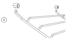
Swing the bottom of the side rack up towards the center of the oven until it is almost horizontal. Slide the prongs at the top out of the mounting slots. Refitting the side racks - main cavity
