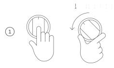
Push in and turn control dial counterclockwise to A. Hold dial at A until A appears in the cooking zone display.
