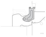
Rotate the locks up into the closed position ensuring they rest inside the slots completely. Note: Incorrect installation will prevent door from correctly sealing.
