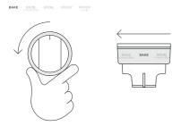
Turn the bezel at the dial's base at any point during cooking to change the function.
