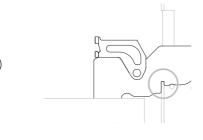
Open the door completely and ensure both hinges are secured by the correct notches.
