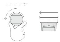
Turn the dial at any point during cooking to change the temperature.
