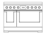
Close the oven door ensuring that when closed, the door is vertical and parallel to any surrounding cabinetry **SELF CLEAN** takes care of the mess and grime that is traditionally associated with oven cleaning. The extremely high temperature of the self-clean cycle burns off and breaks down grease and grime deposits. All that is left is a small amount of ash that can easily be wiped up.
