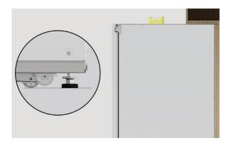
**3.** Prior to installing in alcove, adjust rear feet to the desired height
