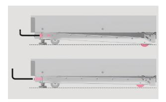
**5.** Lower the rear wheel to achieve clearance between rear feet and floor.
