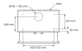
Fig.1 Mounting to underside of cabinetry
