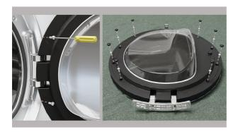
1. Unscrew hinge, remove door and place face down on a protected surface.
