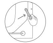
Pull out the two transit rods located below the two lower transit bolt holes. Remove the yellow safety clip from the power cord.
