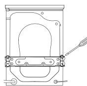
Remove the 4 transit brace screws from the left and right sides of the transit brace.
