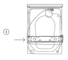
Detach the drain hose from the plastic clasp. Remove the clasps from the left and right sides of the transit brace.
