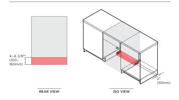
Service outlet at rear extends both sides, hoses and cords can be routed to either or both sides.
