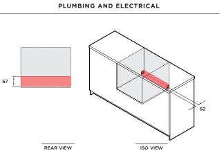
Service outlet at rear extends both sides, hoses and cords can be routed to either or both sides
